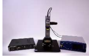
Radiant Tester and Polytec VibroOne Laser
